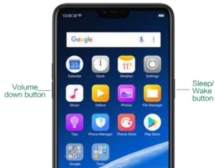
Press and hold the Power and Volume Up buttons: If the phone isn't responding, press and hold the button combination for at least eight seconds to force restart your phone.
